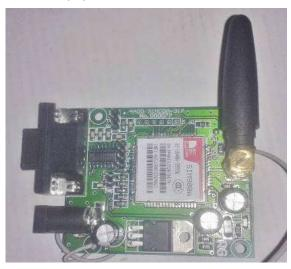
The SIM900 is a complete Quadband GSM/GPRS
