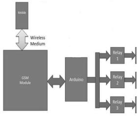
As seen above, we send an SMS from a mobile device, through the GSM network, to the GSM Module present in the automation system.
