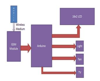
The most basic command is "AT", if GSM respond OK then it is working good otherwise it respond with "ERROR". There are various AT commands like ATA for answer a call, ATD to dial a call, AT+CMGR to read the message, AT+CMGS to send the sms etc. AT commands should be followed by Carriage return i.e. \r (0D in hex), like "AT+CMGS\r". We can use GSM module using these commands.
