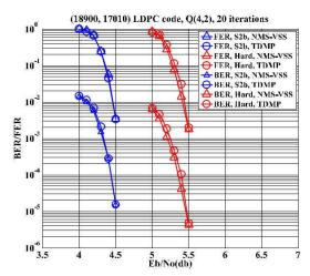
flash memory. The gate count is reported as 520k gates as we resynthesis the postlayout net-list (including SRAMs). Fig. 13 shows the place-and-route result and gate count of major modules. The FER and BER performances over AWGN channel are provided in Fig. 11.
