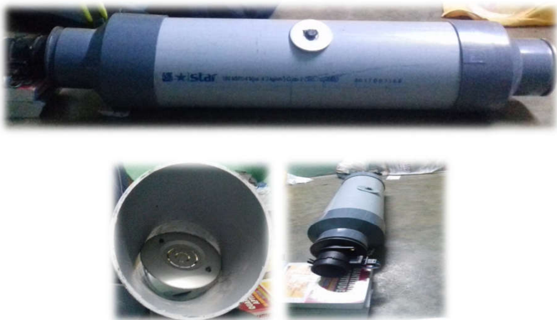
Fig No: 01.1 Wind tunnel witch relative hot wire anemometer
